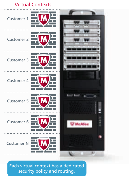
Figure 1. A single master McAfee Next Generation Firewall may be deployed with multiple McAfee Virtual Contexts. Firewall/VPN, intrusion prevention systems (IPS) and level 2 firewall roles are supported.
